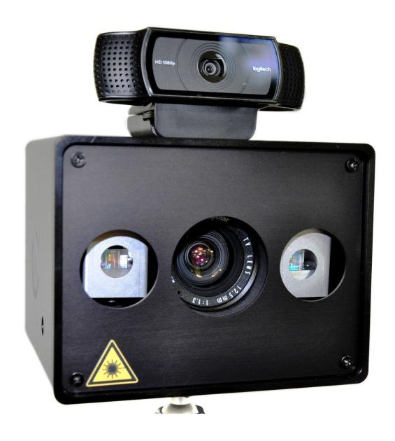
LiDAR OWL – the time-of-flight imaging camera, that could be used with the
