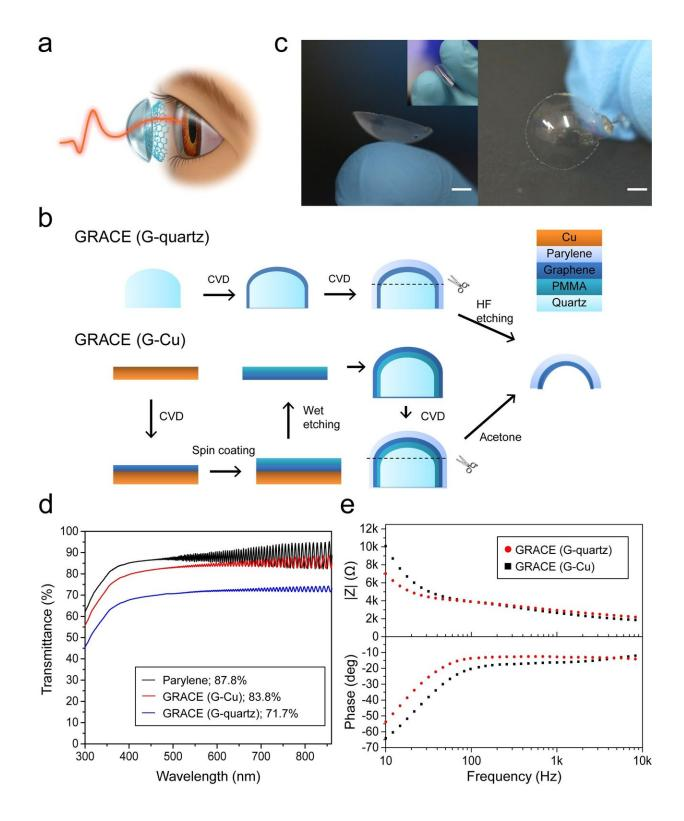
**Fig. 1** GRACE device fabrication and characterization. **a** Schematic drawing of ERG recording with the GRACE device. **b** Schematic illustration of GRACE fabrication with G-quartz and G-Cu. **c** Photographs of a GRACE device made
