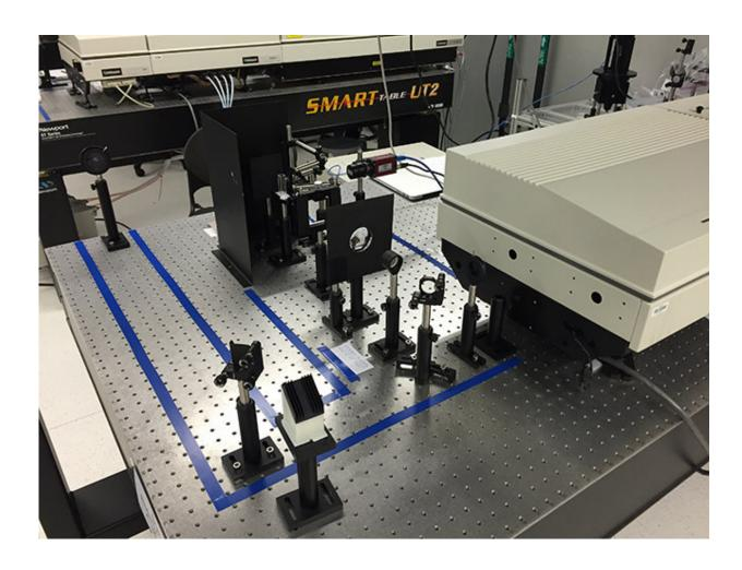
A complex set-up of lenses and cameras are required for direct, laser-based NOx measurements in a flame. Credit: © 2018 Miles Bohon
