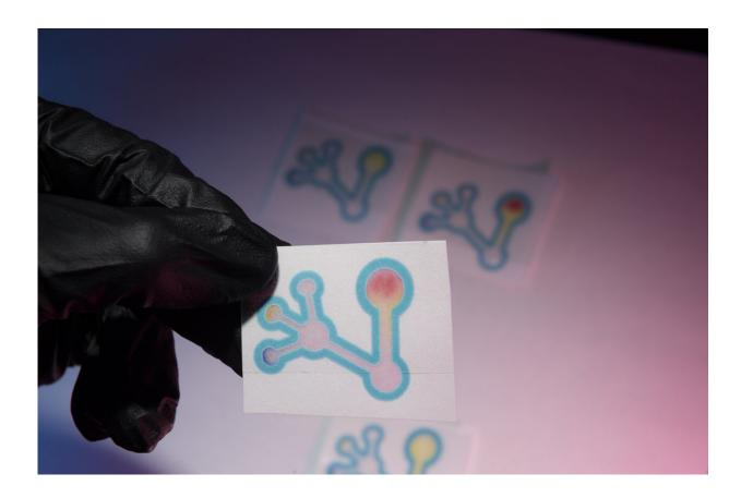
A simple, paper-based test can quickly identify a falsified or substandard antibiotic. Credit: John Eisele/Colorado State University
