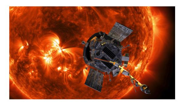
This image made available by NASA shows an artist's rendering of the Parker Solar Probe approaching the Sun. It's designed to take solar punishment like never before, thanks to its revolutionary heat shield that's capable of withstanding 2,500 degrees Fahrenheit (1,370 degrees Celsius). (Steve Gribben/Johns Hopkins APL/NASA via AP)
