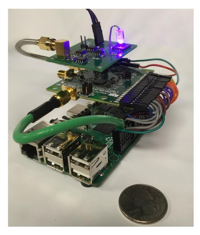
Development of ORNL's quantum random number generator began with basic components including an LED light, the source from which a field of quadrillions of photons are produced. The device can detect and measure the quantum statistics of photons present in the field and use each one as the basis
