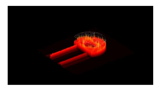
The D-shaped cavity producing quantum chaos within the cavity, and a more stable laser resulting. Credit: Bittner et al.
