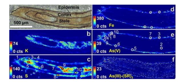
The same section of a P. juliflora plant root revealed by a light-microscope (a) with dotted lines delineating the parts of the root, and XRF imaging (b-f). The color intensity corresponds to the fluorescence signal produced by each chemical component in the sample: potassium (b), sulfur (c), iron (d) and two different arsenic species (e and f). Credit: SLAC
