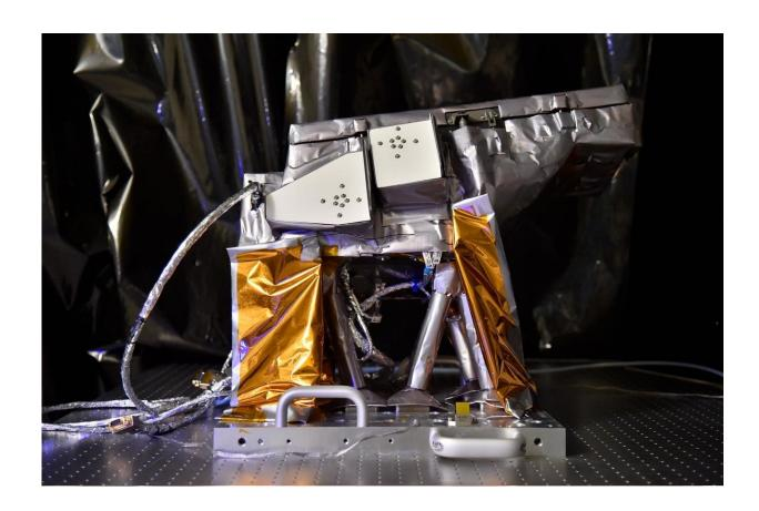
The US Naval Research Laboratory's Wide-Field Imager for Solar Probe, or WISPR, will launch aboard NASA's Parker Solar Probe Aug. 11, 2018. Credit: US Naval Research Laboratory/Jamie Baker
