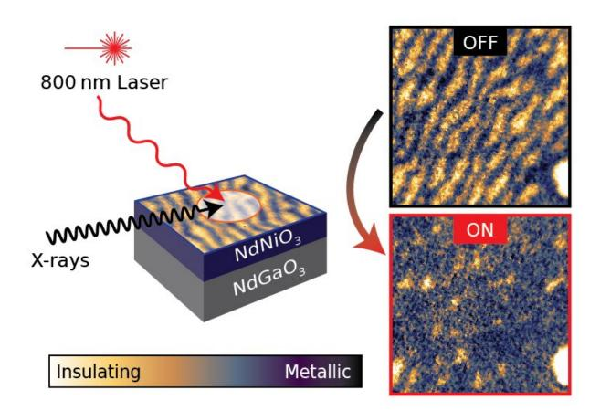
Sending a very fast, high energy pulse of laser light raised the temperature of a sample of neodymium nickelate from 150 to 152 Kelvin for a small instant of time. This small temperature increase was enough to change the property of the material from insulating to conducting. Credit: Giordano Mattoni/TU Delft
