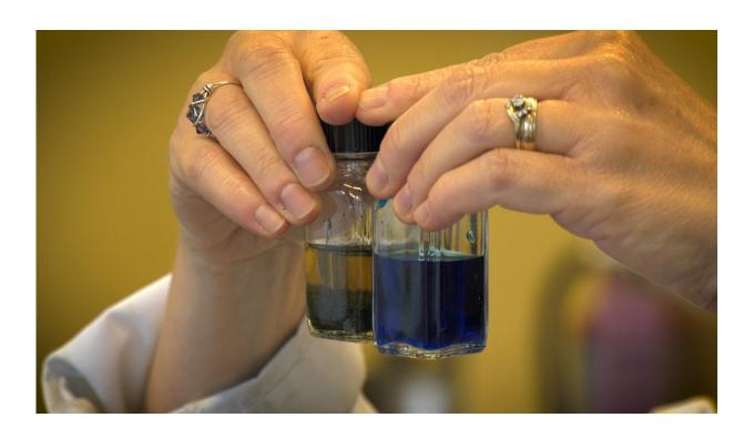
Within hours, dried and ground avocado peels help remove methylene blue dye from water through a process called adsorption. Credit: Dickinson College
