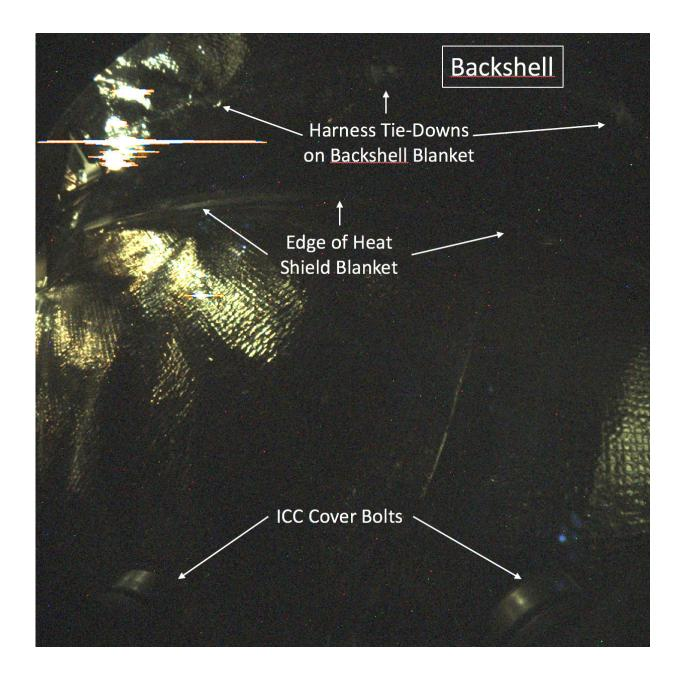
This long-exposure image (24 seconds) was taken by Instrument Context Camera (ICC) of NASA's InSight Mars lander. The image shows some of the interior
