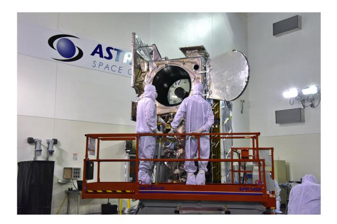
The ICESat-2 satellite undergoes tests one last time before it is placed in the rocket. ICESat-2, scheduled to launch Sept. 15, will precisely measure the height of Earth's ice and monitor change. Credit: USAF 30th Space Wing/Timothy Trenkle
