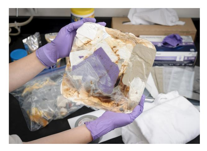
A sample trash tile, compressed to less than one-eighth of the original trash volume, was produced by the Heat Melt Compactor. Credit: NASA/Ames Research Center/Dominic Hart
