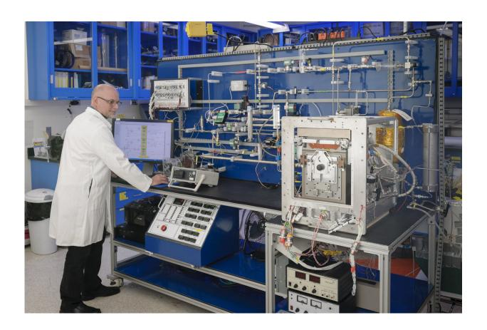
A potential trash management system for future, long-duration space missions, the current version of the Heat Melt Compactor, seen here in its ground configuration, has been tested extensively at NASA's Ames Research Center. Credit: NASA/Ames Research Center/Dominic Hart
