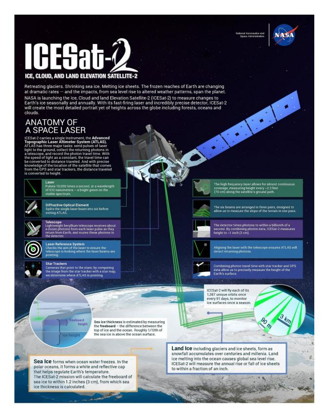
NASA's Ice, Cloud and land Elevation Satellite-2 (ICESat-2) will measure height
