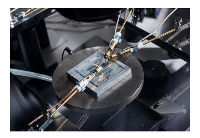
Image shows organic-thin film transistors with a nanostructured gate dielectric under continuous testing on a probe station. Credit: Rob Felt, Georgia Tech
