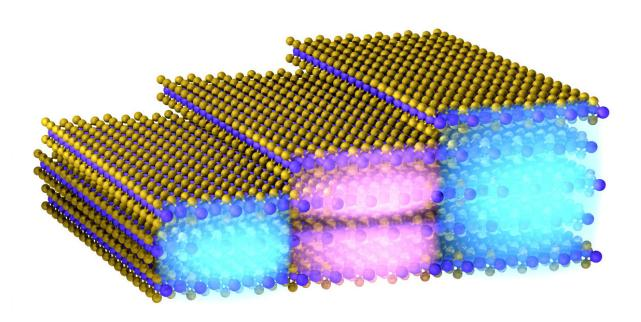
Schematic illustration of charge carriers confined within a TMD flake comprising different thicknesses. Charge carriers in the ground state (blue) can be excited upon resonant light excitation to a higher state (pink). Credit: ICFO/Fabien Vialla
