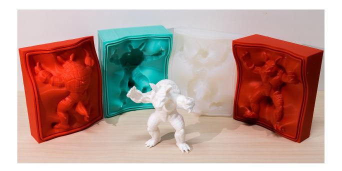
The metamolds (red pieces far left and right) are used to fabricate the silicone molds (greenish and white shapes in the middle). The silicone can then be used repeatedly to form replicas (front). Credit: Luigi Malomo
