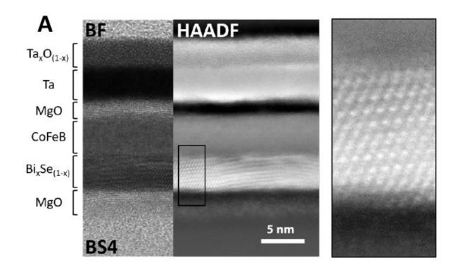
This cross-sectional transmission electron microscope image shows a sample used for the charge-to-spin conversion experiment. The nano-sized grains of less than 6 nanometers in the sputtered topological insulator layer created new physical properties for the material that changed the behavior of the electrons in the material. Credit: Wang Group, University of Minnesota
