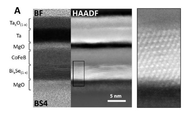
This cross-sectional transmission electron microscope image shows a sample used for the charge-to-spin conversion experiment. The nano-sized grains of less than 6 nanometers in the sputtered topological insulator layer created new physical properties for the material that changed the behavior of the electrons in the material. Credit: Wang Group, University of Minnesota
