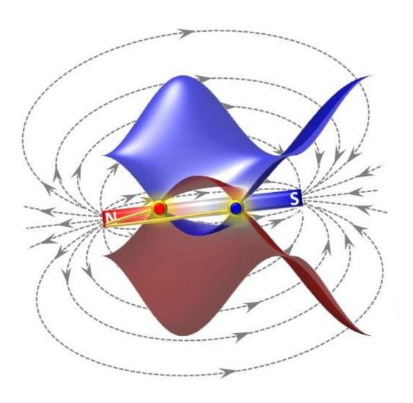
Weyl semimetal with time reversal symmetry broken. The red and blue spheres represent one pair of Weyl points with opposite chirality, which are generated by the intrinsic magnetic moment. The yellow curve is the Fermi arc terminated at this pair of Weyl points. The magnetic moments are schematically described by the magnetic field. Credit: MPI CPfS
