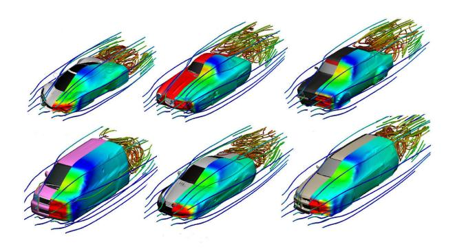
The new software instantly shows stream lines as well as pressure on the surface (color-coded) of interactively deformable shapes. Credit: Nobuyuki Umetani
