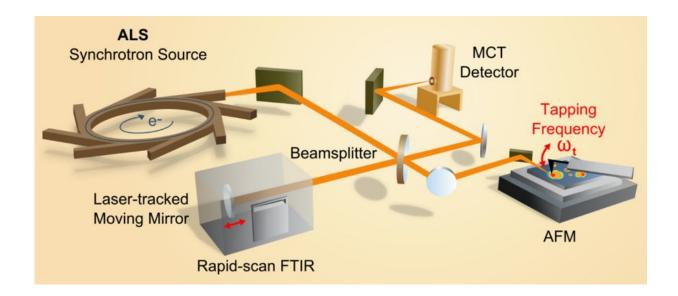
To improve infrared cell-identification to tens-of-nanometers resolution, researchers plan to adapt a synchrotron infrared nanospectroscopy (SINS) system, shown above. The system incorporates highly focused infrared light produced by the Advanced Light Source (integral to "rapid-scan FTIR" or Fourier-transform infrared spectroscopy) and a technique known as atomic force microscopy (AFM). Credit: Berkeley Lab
