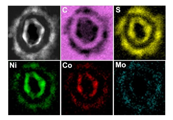
Elemental mapping confirmed sulfur (yellow), nickel (green) cobalt (red) and molybdenum (blue) formed the inner and outer layers, sandwiching an organic layer rich in carbon (pink). Credit: King Abdullah University of Science and Technology
