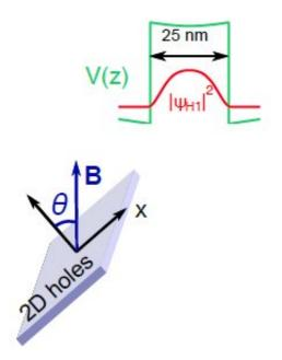
Upper right GaAs hole quantum well used in the study. Lower left: device is tilted at an angle to applied magnetic field. Credit: FLEET
