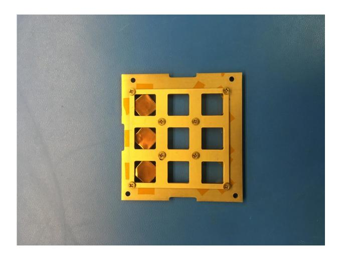
A team led by Professor Barbaros Özyilmaz from NUS CA2DM coated a single layer of graphene on a substrate, and the experiment was placed in the payload enclosure of the 'Wayfinder - Mini' CubeSat. Credit: Boreal Space
