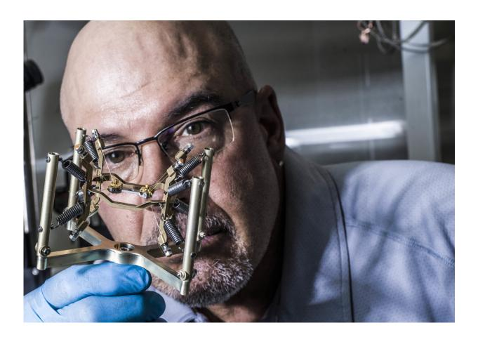
Aptly named a 'Spider' for its eight thermally isolating Kevlar fibers and coiled shock reducing legs, the device pictured here is designed to securely guide small cooling and exhaust tubes throughout the observatory. Credit: NASA/Chris Gunn
