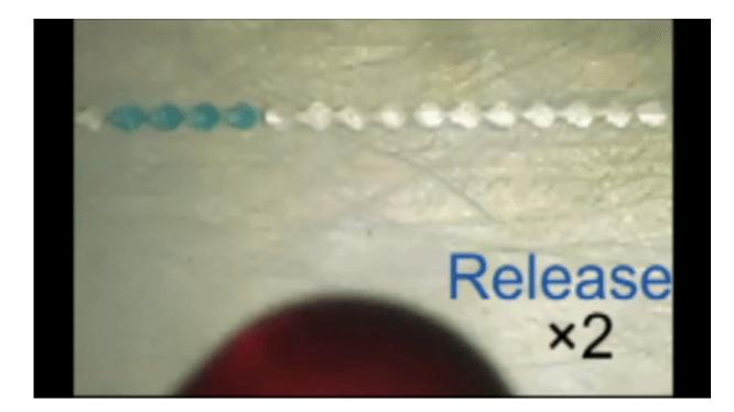
Observing the relationship between the droplet position and the timing of negative pressure applied to control the position of droplets at the level of the single-pixel. Credit: Microsystems and Nanoengineering, doi: 10.1038/s41378-018-0018-1
