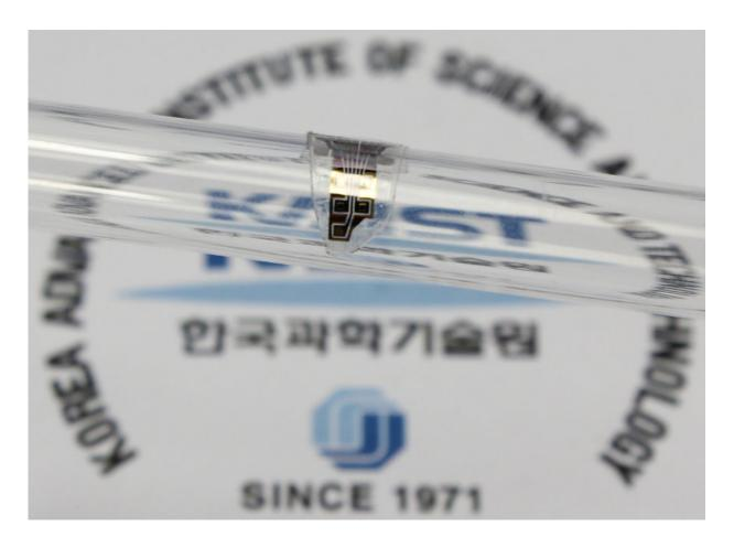
The flexible drug delivery device for controlled release attached on a glass rod. Credit: KAIST
