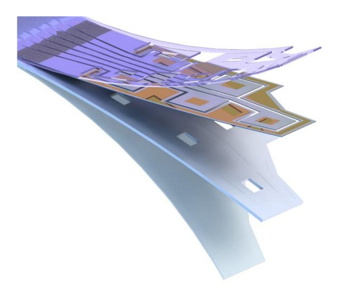
The flexible drug delivery device for controlled release fabricated via inorganic laser lift off. Credit: KAIST
