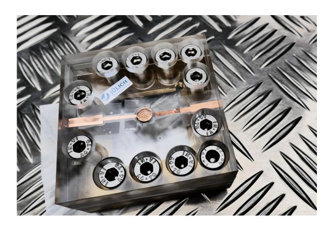
Test set-up for the solid-state battery: the battery of the size of a button cell is located in the middle of the acrylic glass casing, which ensures permanent contact with the battery. Credit: Forschungszentrum Jülich / Regine Panknin
