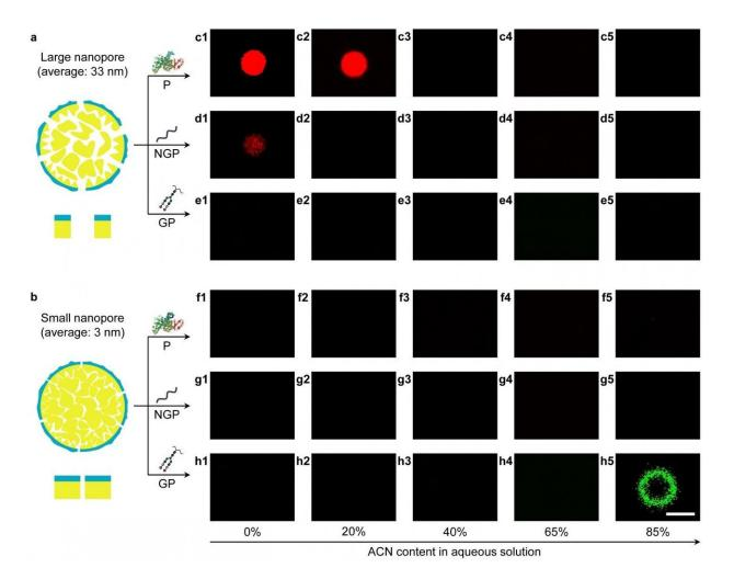
Solvent-switched biomolecule adsorption by the particles with heterostructured nanopores Credit: Dr. SONG Yongyang
