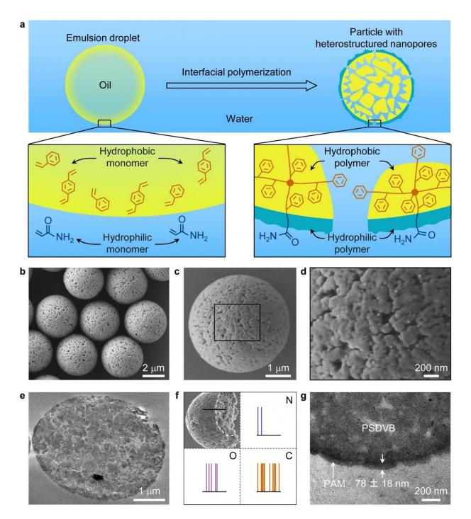
Interfacially polymerized particles with hydrophilic-hydrophobic heterostructured nanopores Credit: Dr. SONG Yongyang
