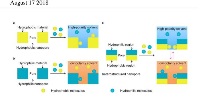
a) Conventional hydrophobic porous materials. b) Conventional hydrophilic porous materials. c) Porous materials with hydrophilic-hydrophobic heterostructured nanopores. Credit: Dr. SONG Yongyang
