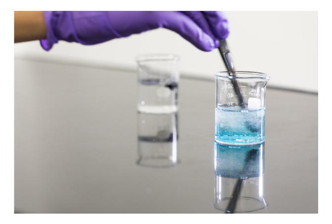
Researchers hold a small piece of the sponge-like material in water containing blue dye. After about 10 seconds, the water in the beaker turns clear. Credit: Mark Stone/University of Washington
