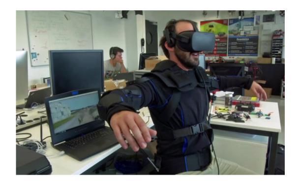
Robotics expert on the Ecole Polytechnique Federal de Lausanne, EPFL team, Matteo Macchini, displays the fly controls in a virtual reality scenario as he controls the flight of a drone, July 23, 2018, in Lausanne, Switzerland. Scientists, engineers and robotics experts at the Swiss university have teamed up to develop a jacket that allows hands-free, torso-controlled flying of drones. (Ecole Polytechnique Federale De Lausanne via AP)
