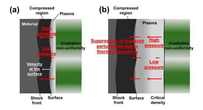
Figure 2. Schematic illustration of laser imprinting. (a) Immediately after laser irradiation. (b) Plasma grows on the target surface with time. Credit: Osaka University
