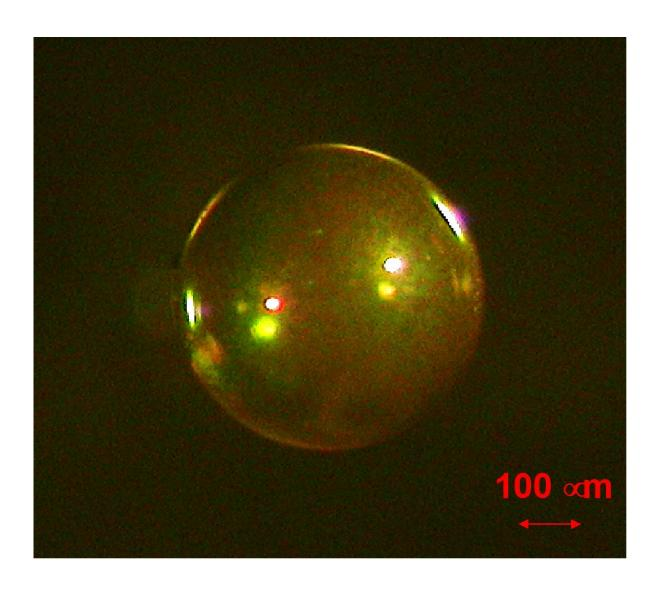
Figure 1. Diamond capsule for nuclear fusion made using the chemical vapor deposition (CVD) method (Diameter:  $\sim 500~\mu m$ , film thickness
