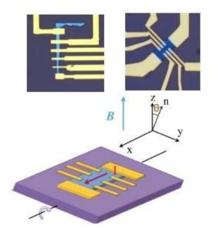
2-D WTe2 samples (upper) and experimental schematic (lower) diagram of angle-dependent measurement configuration. Credit: FLEET
