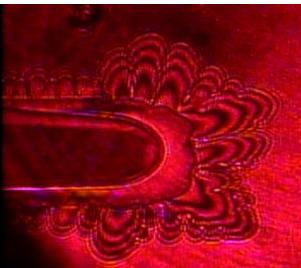
An ice single crystal was visualized simultaneously by bright-field microscopy (left) and Mach-Zehnder interferometry (right) to observe its morphology and growth rates respectively. Credit: Bayer-Giraldi M. et al., *Proceedings of National Academy of Sciences*, July 2, 2018
