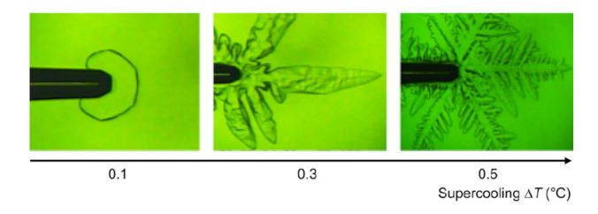
Ice single crystals at different super cooling temperatures observed under a microscope. Credit: Bayer-Giraldi M. et al., *Proceedings of National Academy of Sciences*, July 2, 2018
