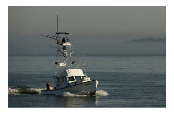
In this Friday, July 27, 2018 photo, a fishing boat equipped with a tuna tower motors out of Casco Bay in South Portland, Maine. The extra elevation of the tower helps fishermen to spot tuna moving near the water's surface. (AP Photo/Robert F. Bukaty)
