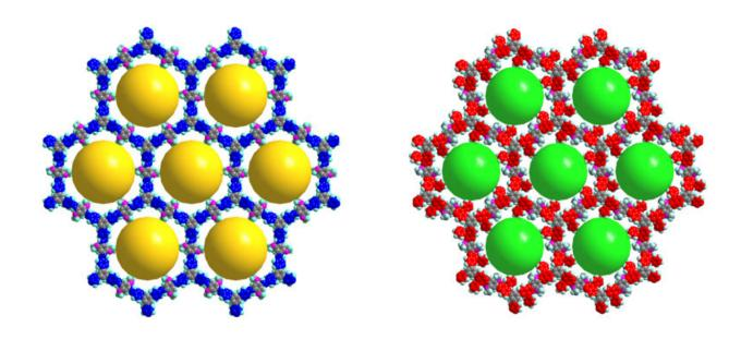
At left is the simulated 3D molecular structure of a covalent organic framework, and at right is a modified framework. The yellow spheres in the structure on the left indicate a pore diameter of 2.9 nanometers, and the cyan spheres in the structure on the right indicate a pore diameter of 2.6 nanometers. Credit: Berkeley Lab
