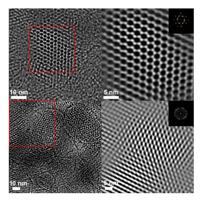
These high-resolution transmission electron microscopy images, produced at Berkeley Lab's Molecular Foundry, show a sheet of covalent organic frameworks (COFs) at the nanoscale (top row), and a sheet of chemically modified COFs (bottom row). Credit: Berkeley Lab
