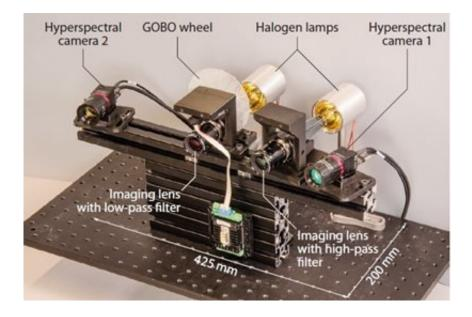
The new hyperspectral imager contains two cameras and measures just 425 by 200 millimeters. With further miniaturization it could be incorporated into smartphones for personal use. Credit: Stefan Heist, Friedrich Schiller University / Fraunhofer IOF
