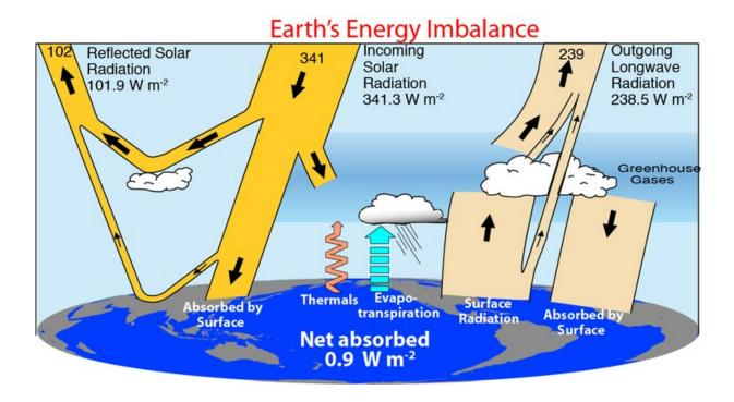
The flows of energy through the climate system are schematically illustrated with numbers on the top-of-atmosphere values and net energy imbalance at the surface. Credit: Trenberth et al 2009
