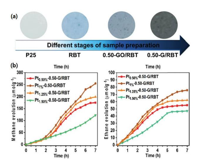
(a) Sample pictures obtained at different stages of synthesis (b) Cumulative methane and ethane evolution for different Pt wt% sensitized 0.50-G/RBT samples. Credit: Daegu Gyeongbuk Institute of Science and Technology (DGIST)
