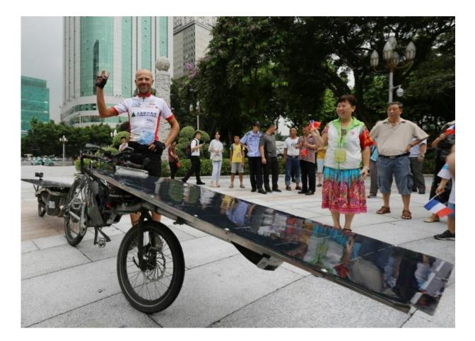
The bike is equipped with two solar panels—one in the front and another on a trailer behind
