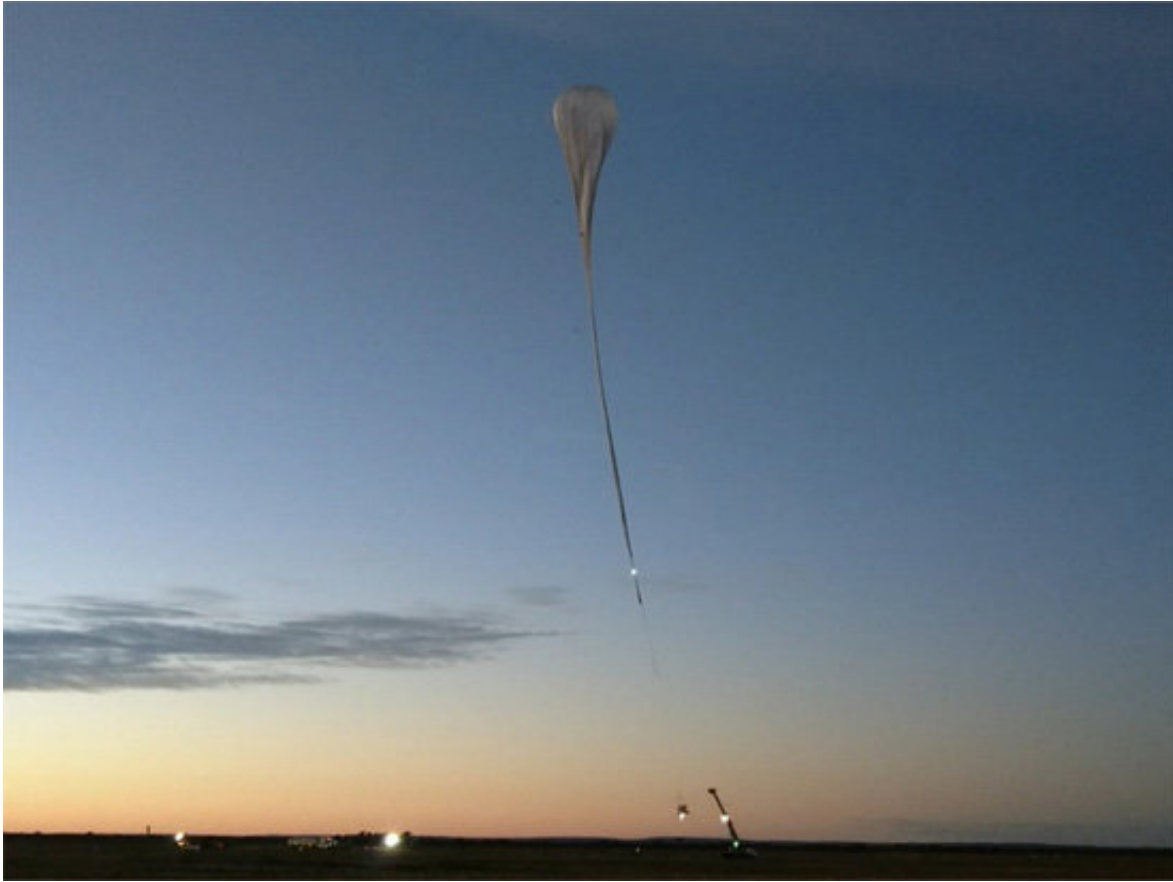
Figure 5: Balloon launch. April 26 at 6:33 local time. The top of the balloon to the bottom (directly above the light) measures 130m. When the balloon is fully inflated it has a volume of 300,000 cubic meters. A parachute and the emulsion telescope (lower light) hang below the balloon, attached by ropes. Credit: Kobe University
