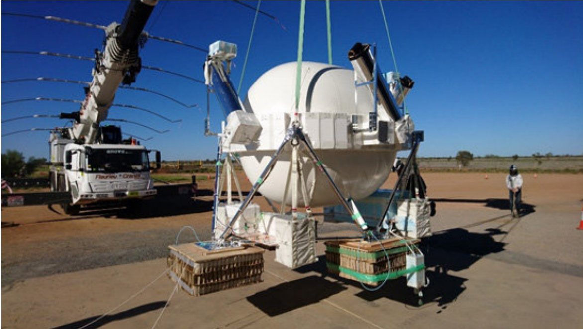
Figure 3: Final preparations for the balloon test. The shell of the pressure vessel is closed. You can see the star camera stray light prevention hoods (silver) pointing in 3 directions. Credit: Kobe University
