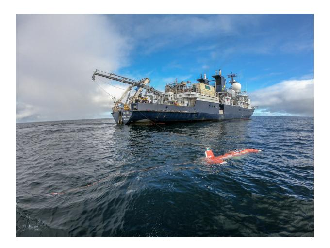
AE2000f is the expedition's scout, it will swim at about 20km/h and collect preliminary images of the seafloor, in order to determine where the rest of the robots should focus. Credit: Schmidt Ocean Institute
