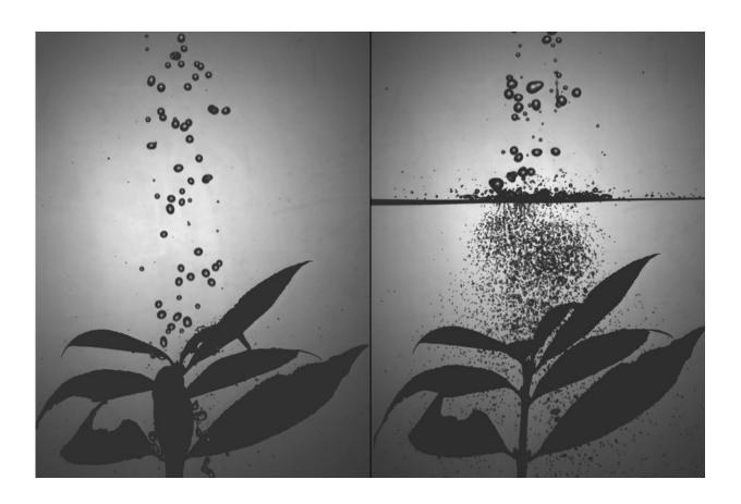
Photos illustrate how the tiny droplets produced by a mesh barrier prevent plants from being pummeled by the larger droplets from either rainfall or the spraying of pesticides, herbicides and fertilizers. The smaller droplets in the image at right have little effect on the plant, while the droplets at left batter its leaves heavily. Credit: The Varanasi Research Group
