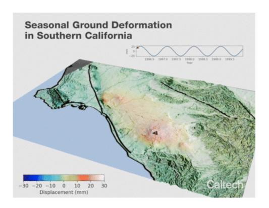
Ground rises and falls as water is pumped in and out of reservoirs—as measured in a study that could impact how municipalities manage this crucial resource. Credit: Bryan Riel and Mark Simons
