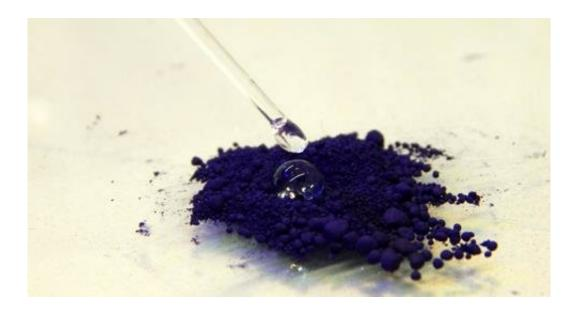
At room temperature the dye indigo is completely water-repellent. A droplet of water easily pearls off. Credit: Vienna University of Technology
