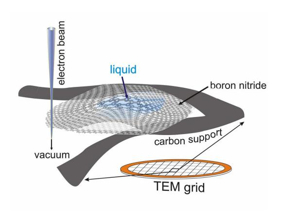
Schematic drawing of the boron nitride cell. Credit: University of Illinois at Chicago
