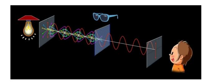
Polarization filters light so that it vibrates in one direction. Credit: Masako Hayashi, CORE-U, Hiroshima University
