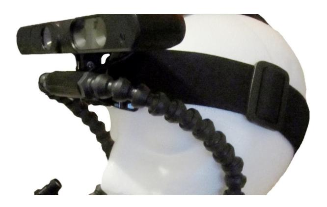
The University of Texas at Arlington has been awarded a patent for a revolutionary new technology that is able to scan a user's eye movements and enable them to navigate mobile platforms, such as electric wheelchairs, without the use of hands. The technology would also allow users to communicate to a robotic platform when they would like to use an object, such as a glass of water. Credit: UTA
