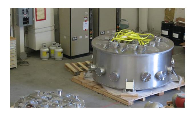
The xenon vessel and vacuum vessel for the next Enriched Xenon Observatory (nEXO) experiment was built at Lawrence Livermore National Laboratory. The experiment will search for an extremely rare nuclear process called neutrinoless double-beta decay (NDBD). Credit: Lawrence Livermore National Laboratory
